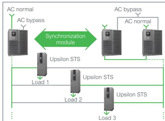
Distribution redundancy with the static transfer switch (Upsilon STS)
